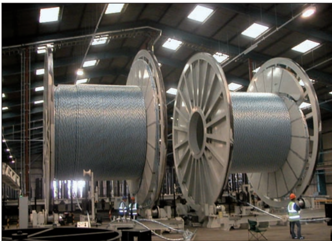
The new JDR facility's 9.2m reels with Greater Gabbard cables.
