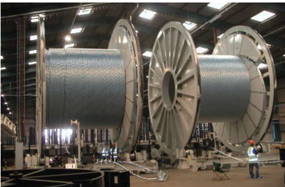
300 tonne / 9.2m diameter process reels.
