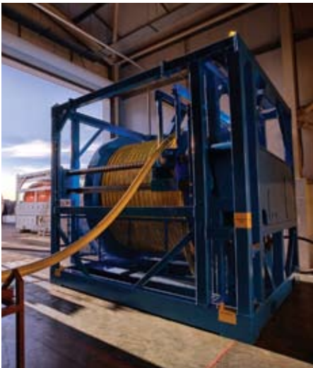
DNV certified workover control reeler system.
