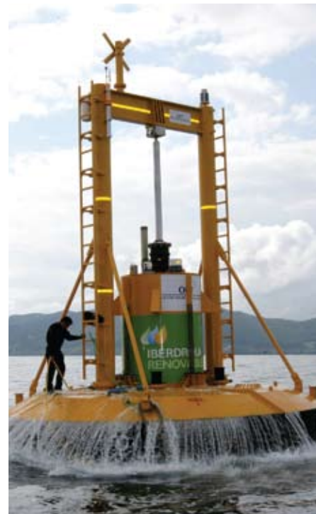
JDR will provide the cable for OPT's PowerBuoy wave energy converter. (photo courtesy of Ocean Power Technologies)
