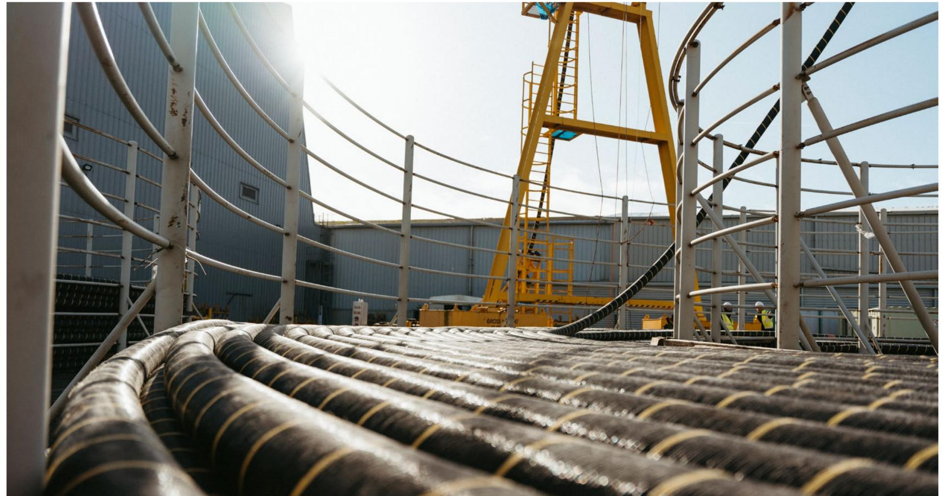
four subsea umbilicals, ranging from 7 km to 48 km in length, connecting steel pipes, medium voltage electrical cores and fibre optic cables. The cables will be manufactured at the JDR plant in Hartlepool, UK. Once completed, umbilicals will be loaded onto a vessel and shipped to Abu Dhabi to the offshore facility.
